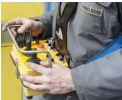
The DOCKMATE ® is operated by portable remote control.
