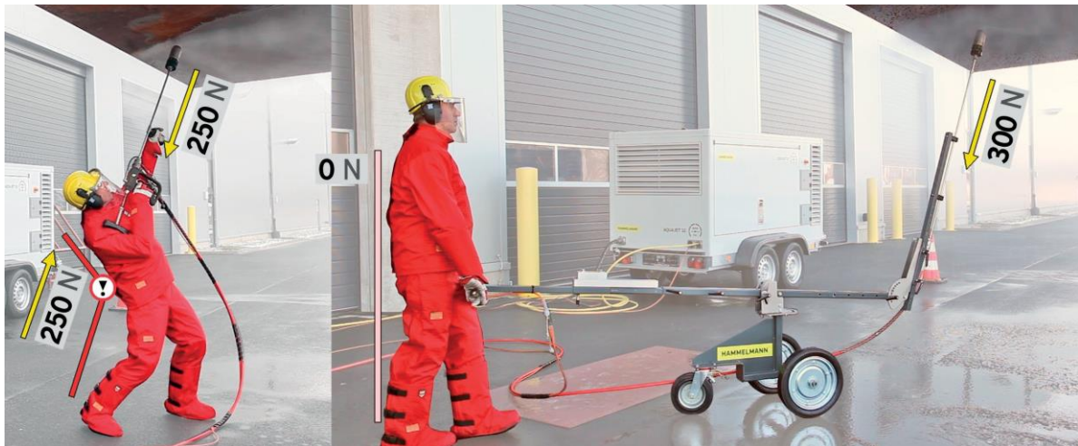
Manual blasting gun work
